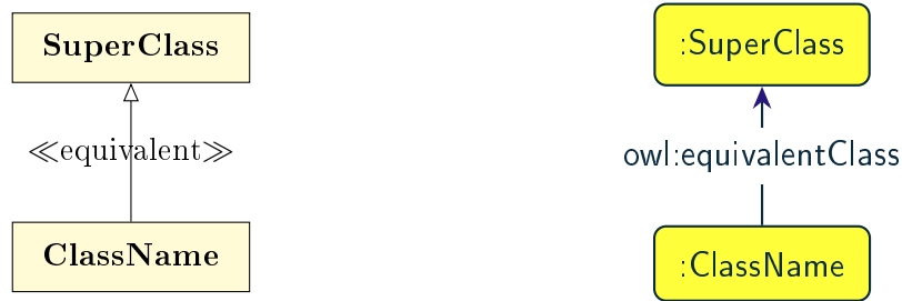
Figure 15: Visual representation of UML class equivalence (on the left) and OWL class equivalence (on the right)
