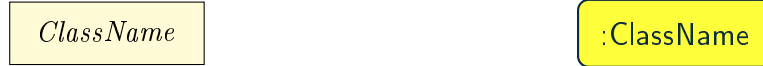
Figure 7: Visual representation of an abstract class in UML (on the left) and OWL (on the right)
